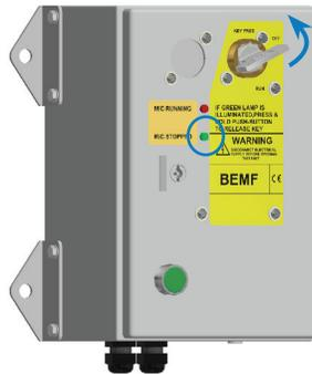
Turn the key to OFF position to switch the power off. A movement detector gives a signal to the BEMF unit once zero movement has been detected. This will illuminate a green LED. The key may now be released by pushing the green button. This key is then taken to unlock the access lock on the motor unit.
