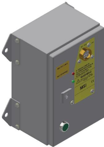
The MSI is designed to control access to rotating machinery that has a run-down time. The MSI relies on the detection of motion via two sensors. Only when both sensors detect zero movement can the key be released. The MSI has been designed to provide high level of safety when installed as part of an access control system for dangerous machinery.
