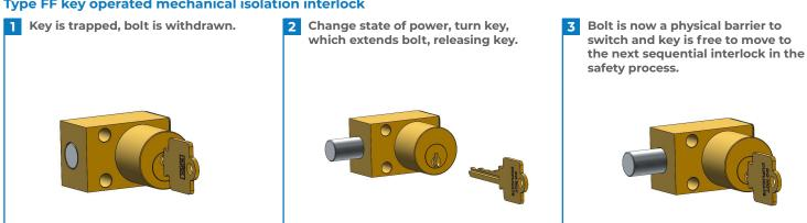
The length of the bolt is available in various lengths to suit each unique application. The travel of the bolt is always 3/4".
