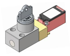
The thermoplastic bodied auxiliary switch provides 2 N/O 1 N/C 5amp or 4 N/O 2 N/C 5 amp contacts that respond directly to the movement of the locking bolt when the key is turned. The contacts change state when the key is turned is a slow-make, slow-break device.
