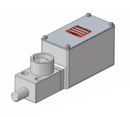
The KIRK K auxiliary switch is a quick-make, quick-break device capable of handling relatively large currents. The toggle switch responds to the movement of the lock bolt as it travels ¾". The Type K switch is a DP/DT switch with ratings of 10A 25VAC/VDC or 15A 15VAC/VDC and is UL Listed and CSA approved.
